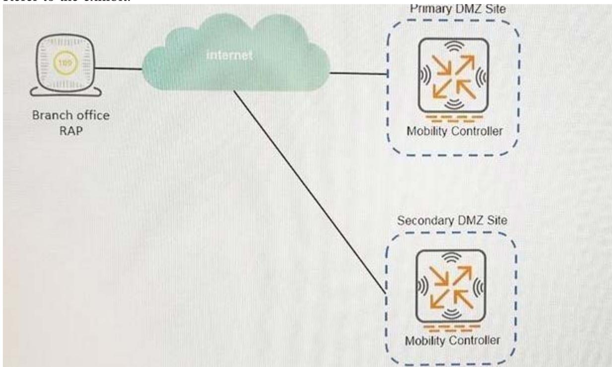
An administrator supports a RAP at a branch office shown in the exhibit. The company has one Mobility Controller (MC) at the Primary DMZ site and one at the Secondary DMZ site. The RAP is configured to connect to only the MC at the Primary DMZ site. A network outage with the ISP at the
