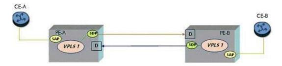
Assume PE-B expects avian tag as part of the RFC 4762 (Martini) encapsulation. How must PE-A be configured?
