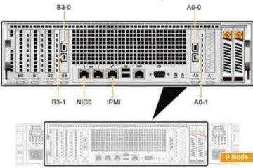
A. Ports AO-1 and AO-1 are connected to the 10GE switch. A back-end network IP address must be planned for each of the two ports.
