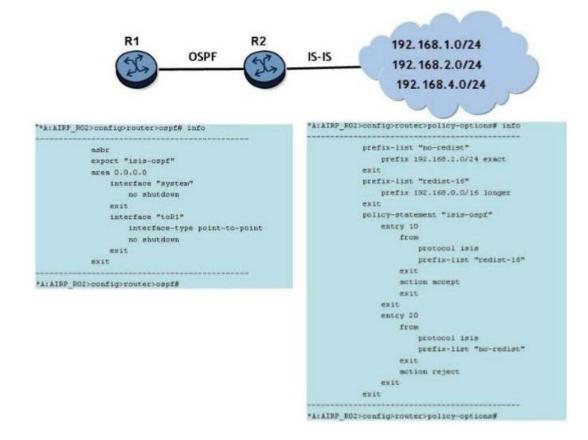
Router R2 learns the networks shown from IS-IS.Router R2 is configured to redistribute routes from IS-IS to OSPF as shown. Assume the OSPF and IS-IS adjacencies are operational.
