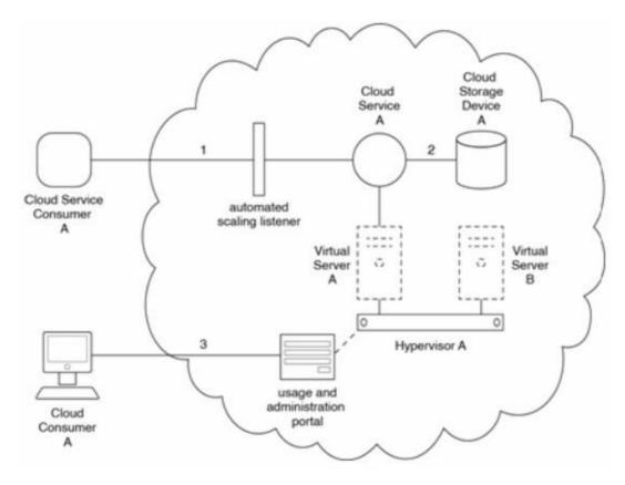
Cloud Service Consumer A accesses Cloud Service A (1), which either sends a query or a read/write request to a database on Cloud Storage Device A (2). A usage and
