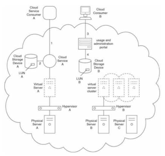
Organization A would like to deploy two of its legacy systems on Virtual Server A and to further extend Cloud Service A's functions so that it can be used as an external interface for cloud service consumers to access legacy system features. Additionally, Organization A would like to deploy three of its mission-critical legacy systems on Virtual Server B in
