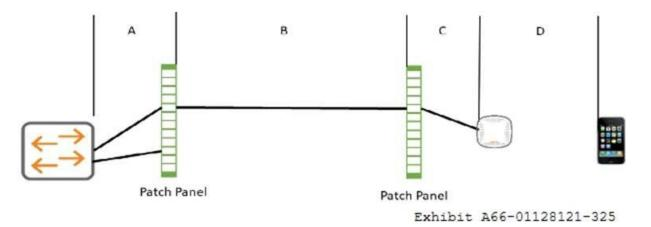
When planning the use of Cat7 cabling for a SmartRate connection between an ArubaOS AP and an ArubaOS switch, which sections should be considered when calculating distance?
