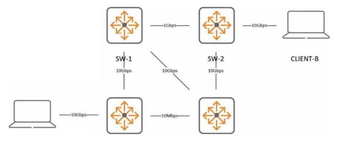
All ports are routed, and ECMP is enabled, with other default parameters for OSPF.
