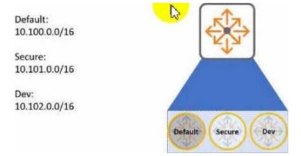
Aruba CX 6300 switch has routes in three different VRFs as per the example above. The user needs to leak routes between VRF Secure and VRF Dev. and also between VRF default and VRF Dev
