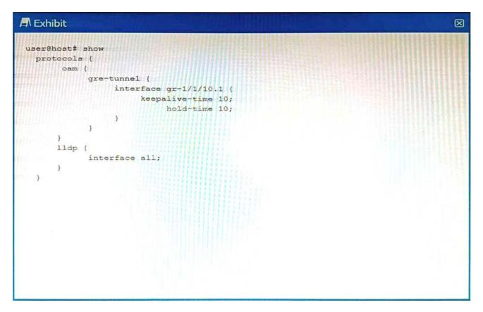
You have configured a GRE tunnel. To reduce the risk of dropping traffic, you have configured a keepalive OAM probe to monitor the state of the tunnel; however, traffic drops are still occurring.
