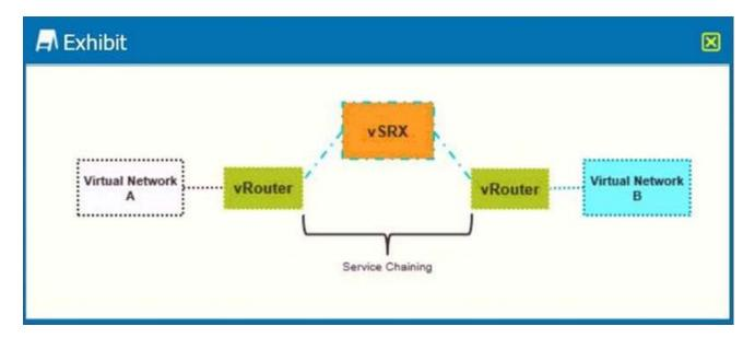
Referring to the exhibit, which statement is true about virtual networks A and B so that the vSRX can be used as a service instance in a transparent service chain?
