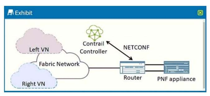
Referring to the exhibit, which role is the router device performing when implementing a PNF service chain?
