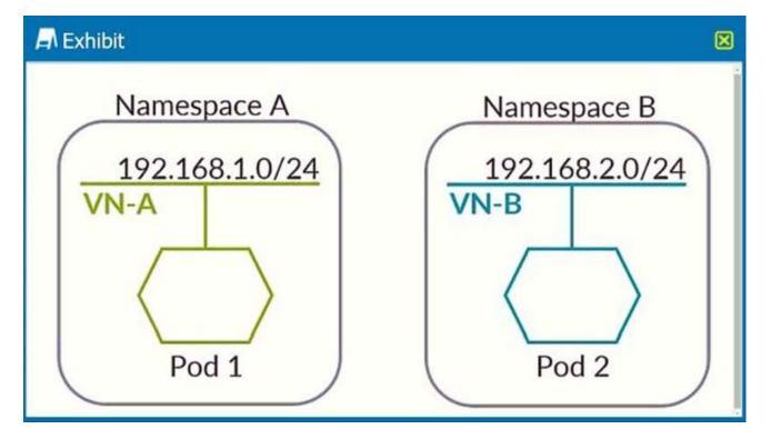
Your company uses Kubernetes as an orchestrator integrated with Contrail. You are asked to create the networks shown in the exhibit and enable communication between Pod 1 and Pod 2.
