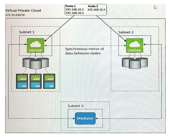
Which deployment model for NetApp Cloud Volumes ONTAP in AWS would use the networking topology as shown in the exhibit?
