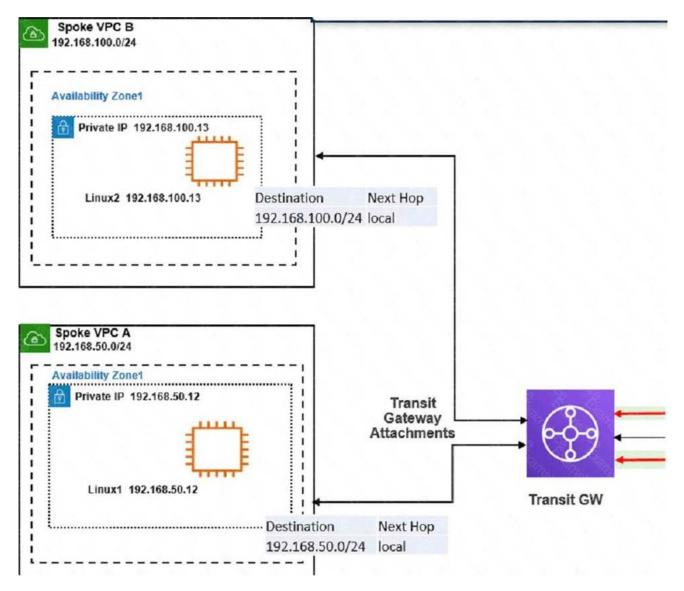
The exhibit shows a customer deployment of two Linux instances and their main routing table in Amazon Web Services (AWS). The customer also created a Transit Gateway (TGW) and two attachments
