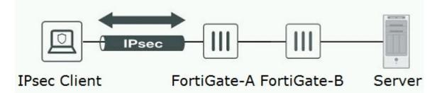
Only users authenticated in FortiGate-B can reach the server. A customer wants to deploy a single sign-on solution for IPsec VPN users. Once a user is connected and authenticated to the VPN in FortiGate-A, the user does not need to authenticate again in FortiGate-B to reach the server.
